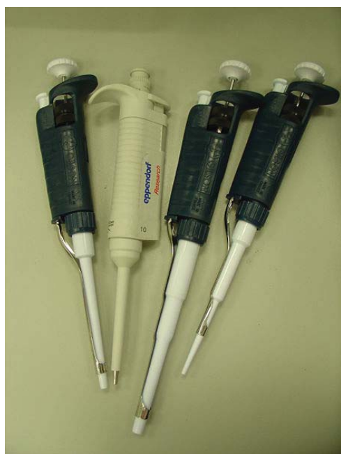
Figure 2.6 Digital micropipets. From the left, the pipets deliver volumes of 50 \mu\text{L} –200 \mu\text{L} ; 0.5 \mu\text{L} –10 \mu\text{L} ; 100 \mu\text{L} –1000 \mu\text{L} ; 1 \mu\text{L} –20 \mu\text{L} . Source: Retama (commons.wikimedia.org).
