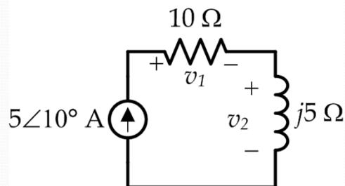
$$S_R = I_S^* \cdot V_1 = (5\angle -10^\circ) \times (50\angle 10^\circ) = 250 + j0$$
