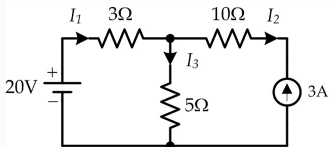
$$KCL: I_1 = I_2 + I_3 \quad I_1 = 0.625 \text{ A}$$
