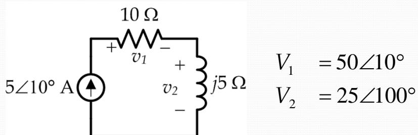
$$V_S = V_1 + V_2 = 56\angle 36.6^\circ$$
