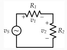
$$v_1 = v_s \frac{R_1}{R_1 + R_2}$$
