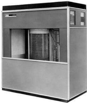
(a) IBM 350 Disk Storage Unit up to 20 MB of storage (1956).
