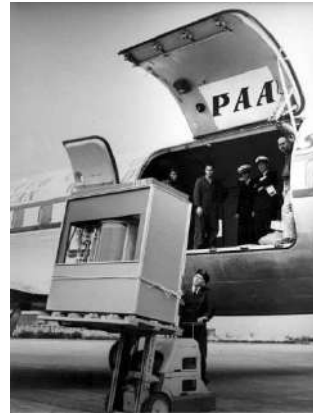
(a) IBM 350 Disk Storage Unit up to 20 MB of storage (1956).
