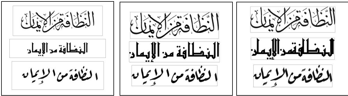
Fig. 4. Examples of text images, before preprocessing (a), after removing the empty rows/columns around the text (b) and between the letters (c).
